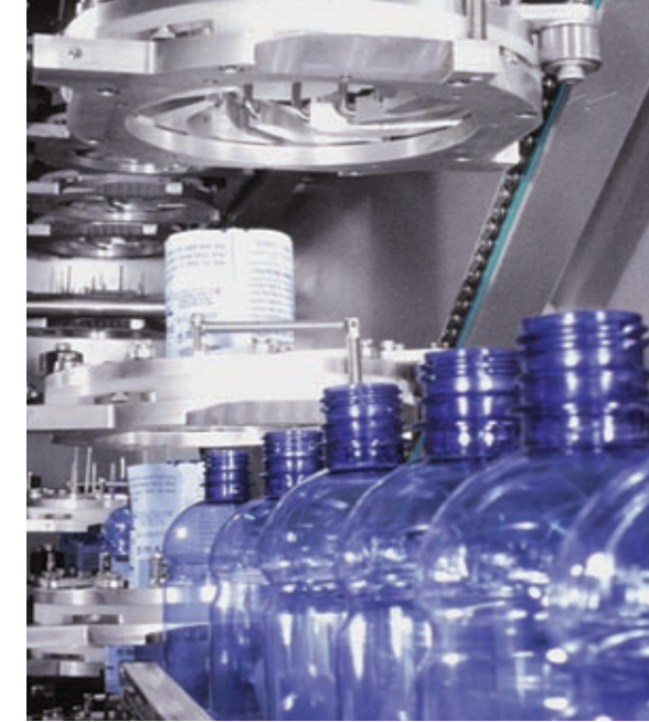
Axon's patented continuous motion machines are capable of processing heat shrinkable and stretch sleeve labels.
